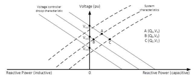
Figure G.1: Voltage droop control and system sharing voltage control at POC
