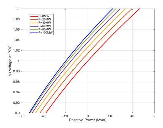
Figure E.4: System V-Q characteristic at POC for various X/R; P=100MW, SCC=400MVA, Vs=1pu
