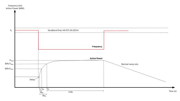
Figure 3-9: Frequency control and hold time demonstration for system over-frequency events; (a) frequency stays outside Frequency Dead Band after 10 seconds of reaching 90% of the final response, (b) frequency stays outside Frequency Dead Band and frequency response sustains after 10 seconds of reaching 90% of the final response, (c) frequency returns to Frequency Dead Band after 10 seconds passes, (d) frequency returns to Frequency Dead Band after 10 seconds passes
