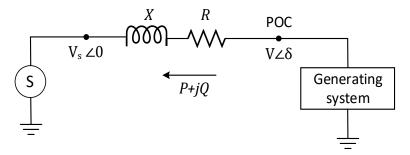
If the centre of the system is controlled at voltage  $V_s \angle 0$  and the POC is controlled at  $V \angle \delta$ , the apparent power transferred to the system at POC can be written as:
