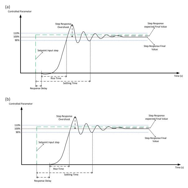
After a step response into a control system, the final step response should settle close to the expected value within a defined error tolerance. A PI controller will always bring the controlled signal to the expected final value; however, the actual response might deviate due to process tolerances. The step response final value might deviate from the step applied if droop control is utilised.
