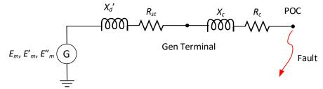
For the faults at the Connection Point, the impedances between generator terminal and the fault location affects the current contribution. For each period, the short circuit contribution of such synchronous machine will be as follows:
