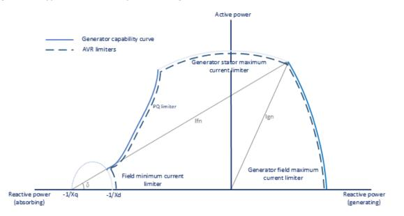
Figure 3-3 Reactive Power capability curve ideal and min requirements
