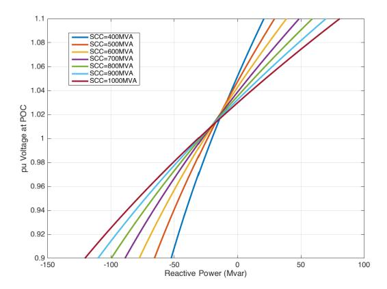
Figure E.5: System V-Q characteristic at POC for various SCC; P=100MW, X/R=3, Vs=1p
