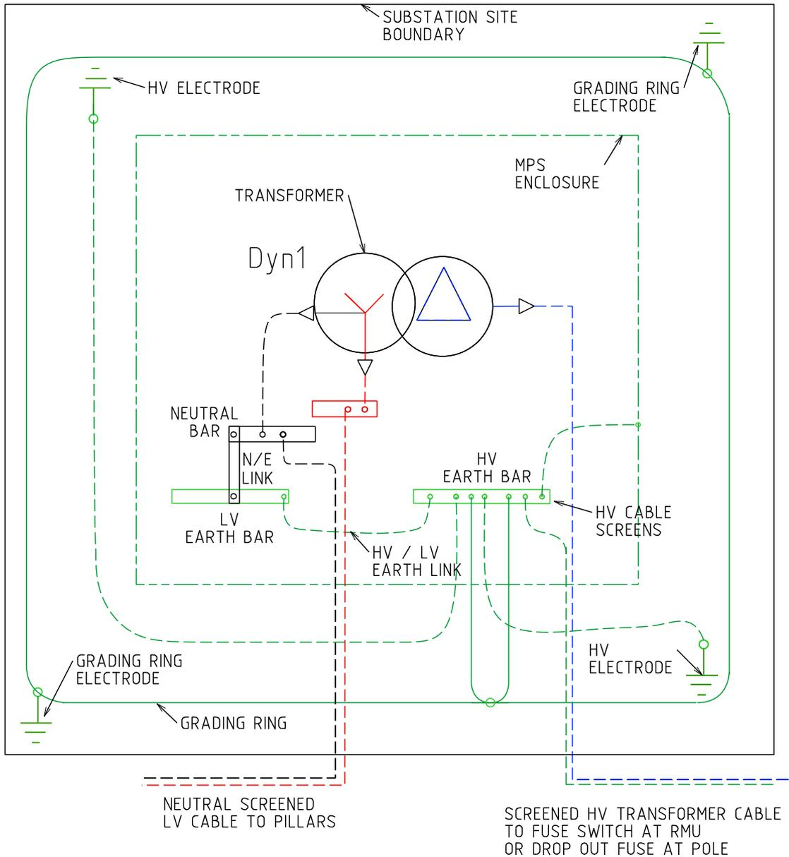
Note that the Modular Packaged Substation (MPS) requires 2 additional electrodes connected to the grading ring. These grading ring electrodes consist of a single 1.5m long earth stake and do not have a target earth resistance.
