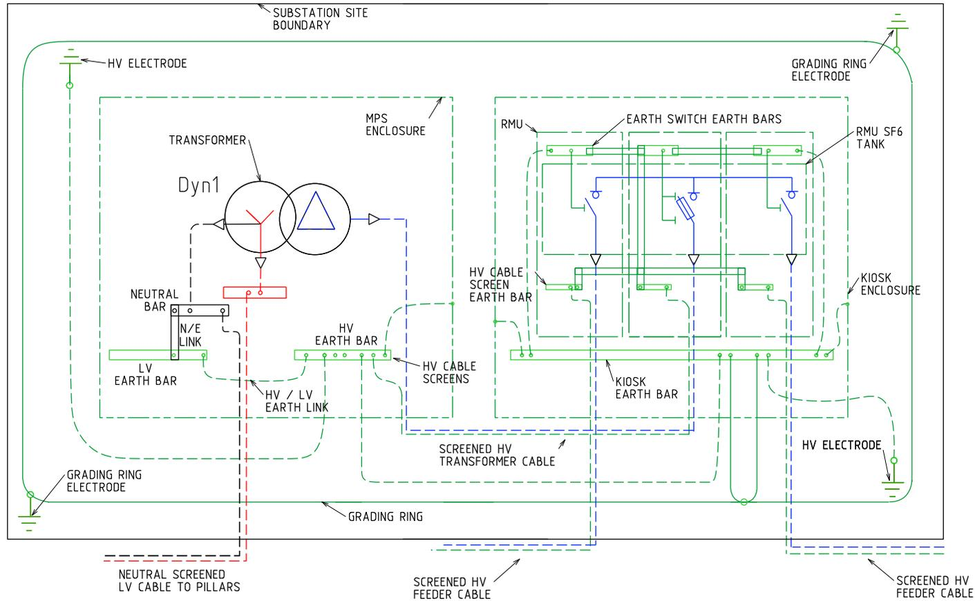
Note that the Modular Packaged Substation (MPS) requires 2 additional electrodes connected to the grading ring. These grading ring electrodes consist of a single 1.5m long earth stake and do not have a target earth resistance
