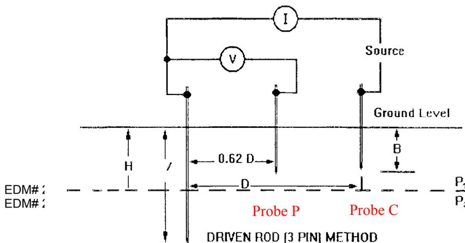
Below is a guide of test lead lengths required to test electrodes of various depths, which should be followed to achieve correct earth resistance readings. The test lead length is not limited to 320m, where the test equipment is capable of longer lengths.
