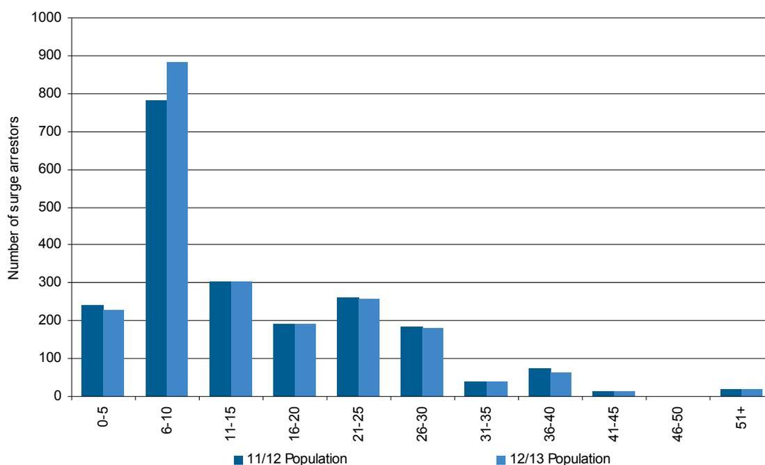
31 surge arrestors (1.4% of the population) have exceeded their design life of 40 years and 149 (6.8%) require mitigation, due to assessed conditions such as insulation degradation, lack of spare parts or component issues.
