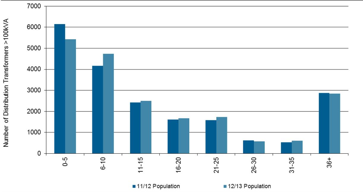
343 distribution transformers (1.7% of the population) have been assessed with conditions requiring their replacement, an increase of 23% from 2011/12. Better and more widespread implementation of the inspection program has increased the defect find rate, with more distribution transformers being identified for replacement during the inspection process and fewer in-service failures. Figure 10 shows the condition profile of distribution transformers.
