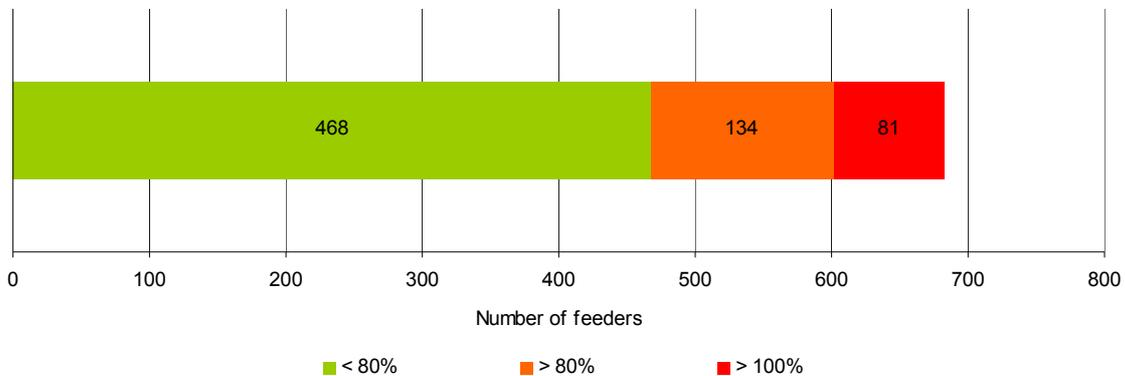
If an overutilised feeder surrounded by other interconnected feeders is subject to an unplanned outage during the summer peak, it may take longer than normal (in excess of two to three hours) to restore supply completely. This is because the entire lost customer base cannot be transferred on to the adjacent interconnected feeders due to a lack of Distribution Transfer Capacity and overutilisation of existing feeders.
