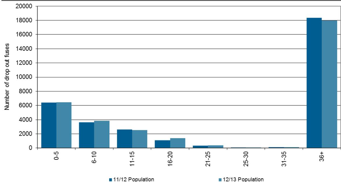
4,636 dropout fuses (14.12% of the population) have been assessed with conditions requiring their replacement, an increase of 47% from 2011/12. A review of the dropout fuse asset strategy resulted in the identification of new failure modes. More dropout fuses are therefore being identified for replacement during the inspection process, reducing in-service failures.
