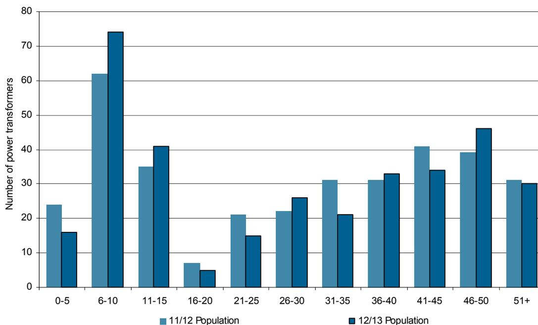
96 power transformers (28.2% of the population) have exceeded their design life of 40 or 50 years (depending on transformer size) and 32 (9.4%) require mitigation independent of their age, due to assessed conditions such as insulation degradation, lack of spare parts and component issues.
