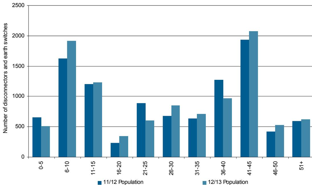
621 disconnectors and earth switches (6.0% of the population) have exceeded their design life of 50 years and 639 (6.2%) require mitigation independent of age, due to assessed conditions such as mechanical degradation, lack of spare parts or component issues.
