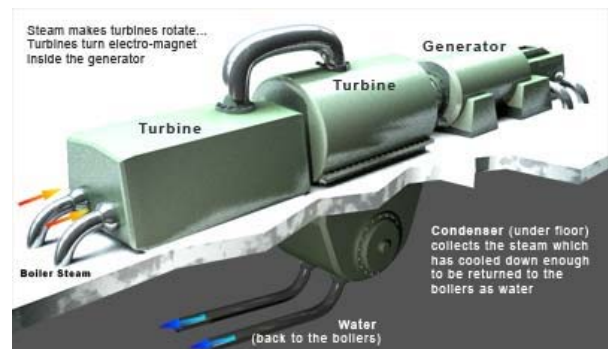
Above - A diagram demonstrating how steam energy is converted into mechanical energy causing the fans in the turbine to spin, thus turning the generator to produce electricity.
