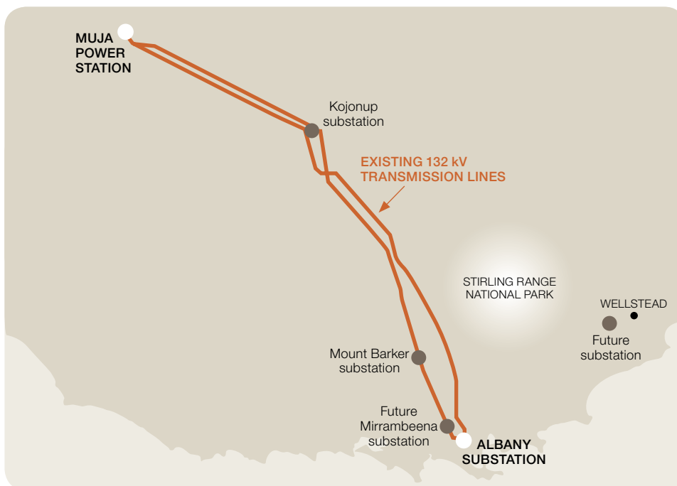
Two existing 132 kV transmission lines between Kojonup and Albany.
