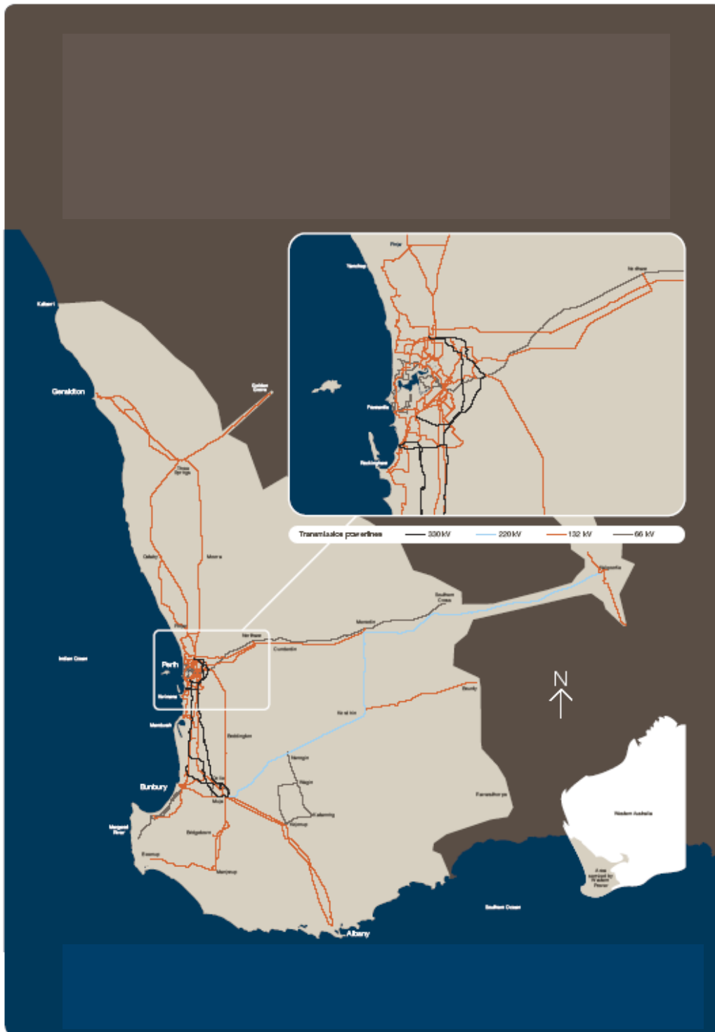
Figure 1 – Western Power's Electricity Network
